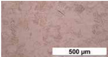
Microstructure of LaserForm Ti Gr5 (A) as built in DMP process without additional stress relief or heat treatments that further improve the structure
