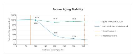
Performed in accordance with ASTM D4329 to simulate ASTM D4459, Indoor exposure of plastics from solar radiation through a window
