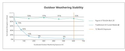
Performed in accordance with ASTM G154 to simulate actual outdoor exposure of plastics
